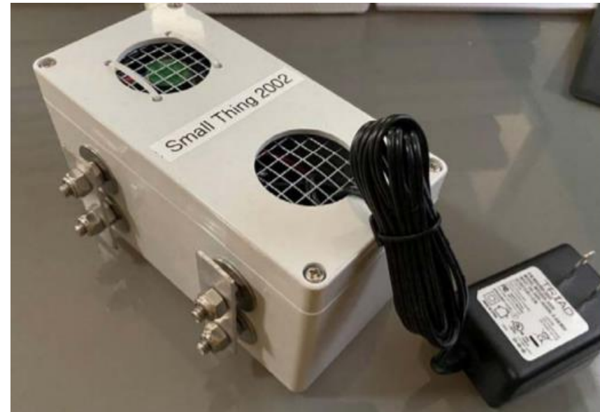
Smart City IoT device – LEaRN air-quality sensor
